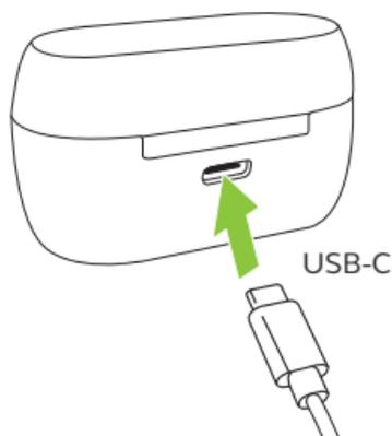
It is recommended to use a power supply with 5V  $\pm$ 0.25V and maximum charging current below 2A. It is not recommended to charge the earbuds or charging case using a power supply with a higher voltage.
